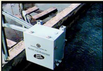
Real time monitor in refinery saltwater discharge canal. Photo courtesy Shell Oil
